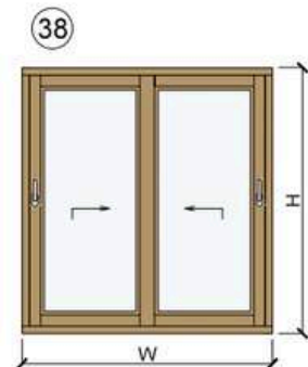
W max=4000 H max 2500 sash weight max 300kg
